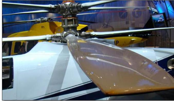
Figure 8 Sikorsky X2 Bearingless Hub
