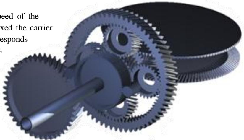
Figure 32 CAD Rendering of Main Rotor Transmission
